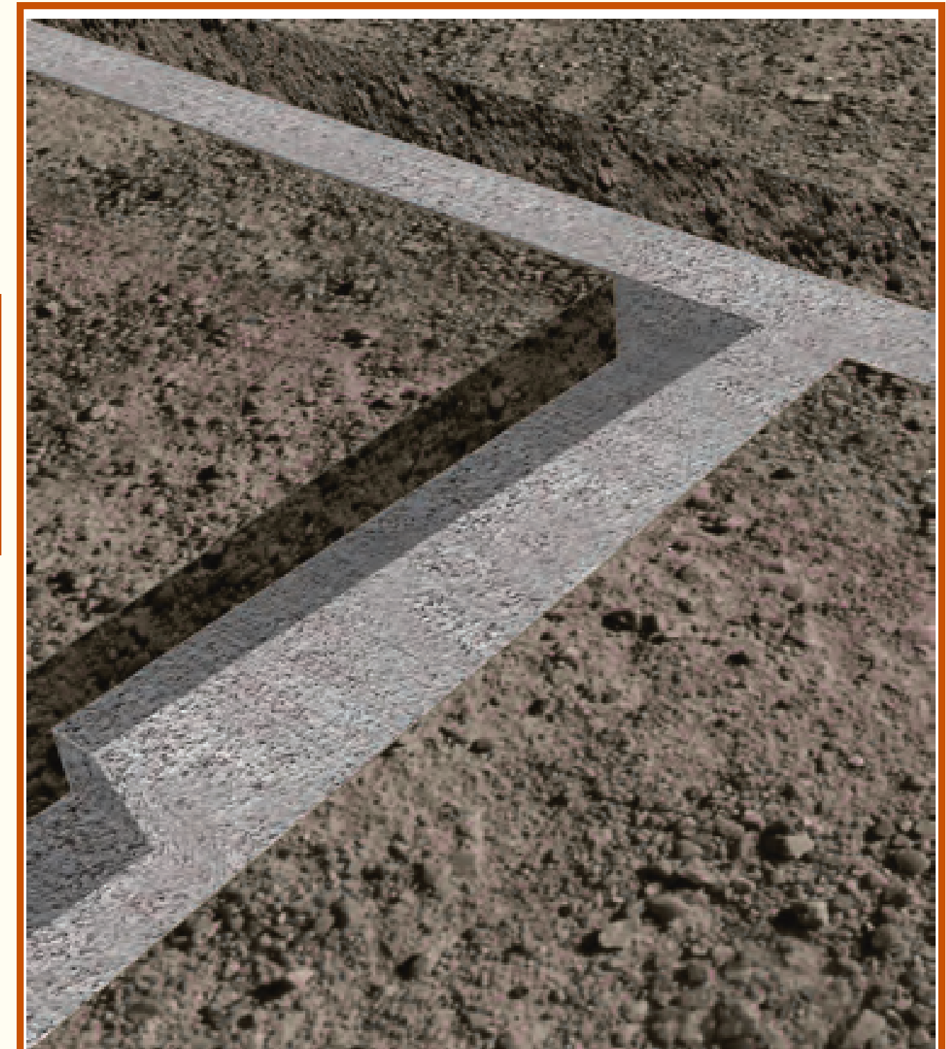
5.19 - Showing completed foundations with steps.
