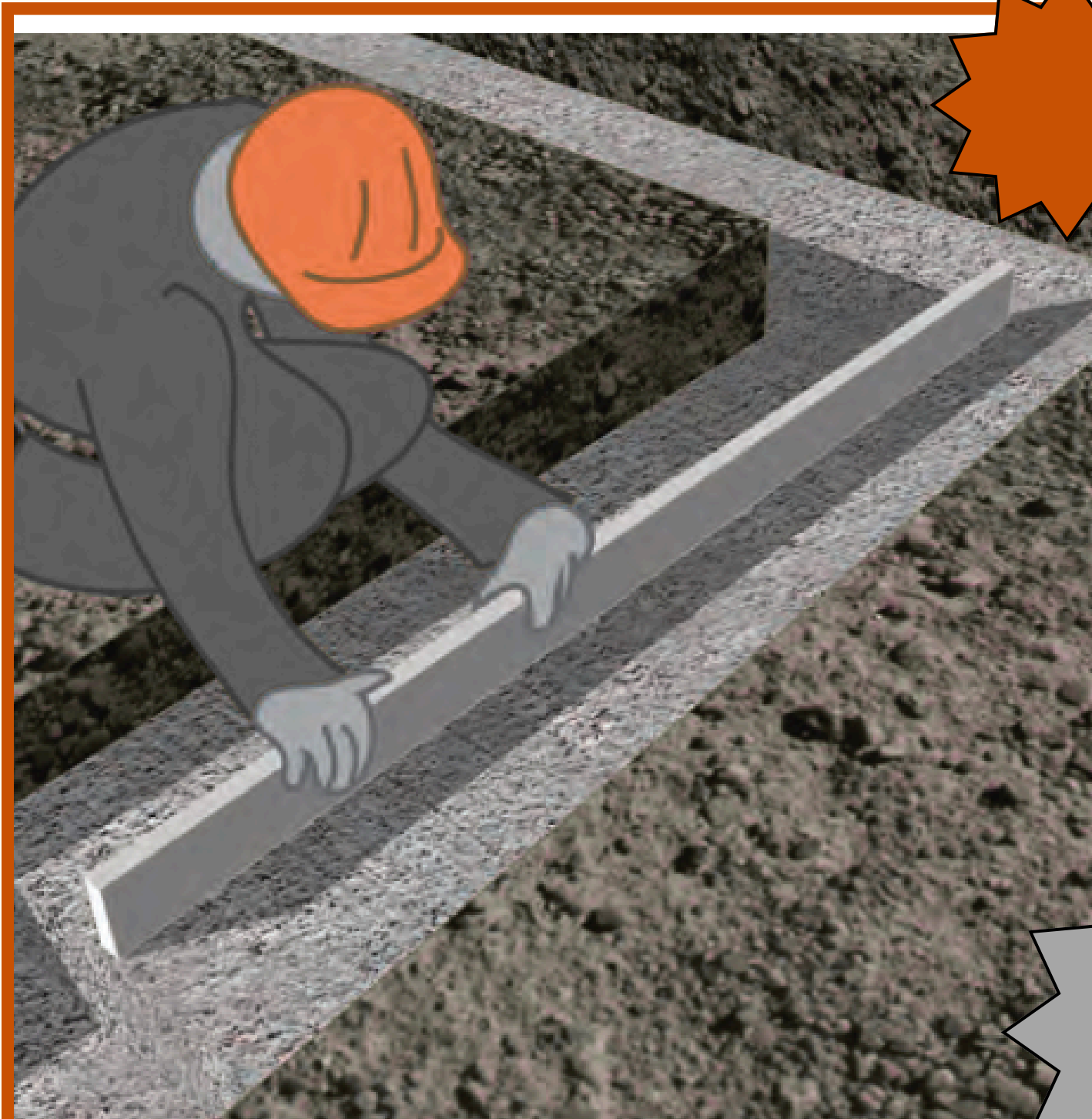
18 - Level the foundation concrete using a straight-edge e top of the concrete thickness pegs.
